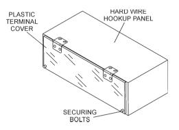
Figure 12. Plastic Face Plate (Output Terminal Lugs)
